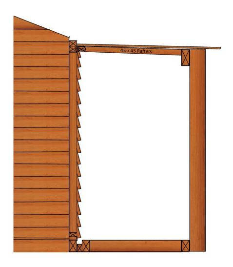
Step 30: Nail Veranda beams and rafters together using 2 x 90mm floor joist nails per join.
