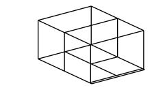
**Step 5:** Carefully roll frame over onto its base. If fitting a Kiwi Floor, fit Floor Joists now. Place the joist centrally and nail in place using three 75mm nails per end.
