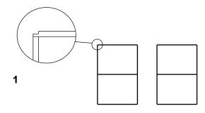
Step 2: Select one 1.715m Base Plate (Green), one 1.715m Top Plate (Red). Stand up End frame with the Stud side of the frame on the ground. Nail 1.715m plates to frame using two nails per join. Ensure Green joins to Green and Red joins to Red. Repeat with other end frame. Position 1.625m Back Wall Nog .883m down from the Top Plate and nail in place.
