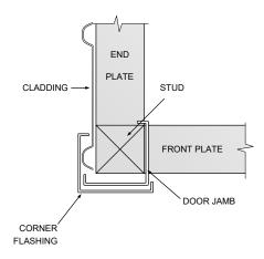
Step 2: On the left hand side of the front wall fit Corner Flashing (101) over Door Jamb Flashing and rib. With top of the Corner Flashing flush with the top of the Top Plate, rivet in place using six rivets.
